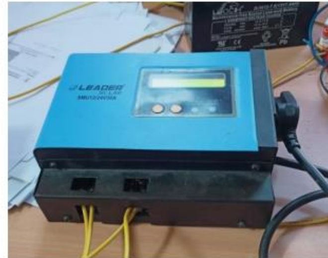
Solar Charge Controller
